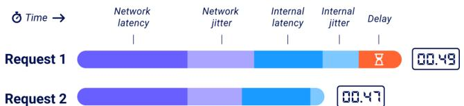
Network jitter is the *variation* in latency - the time taken for a packet to get to a target system and back again. It's the classic nemesis of remote timing attacks. When someone sees a timing attack demonstrated against a local system and says 'That'll never work on a remote system', they're basically saying that network jitter is going to make the attack impossible. Five years ago, this might have been true.
