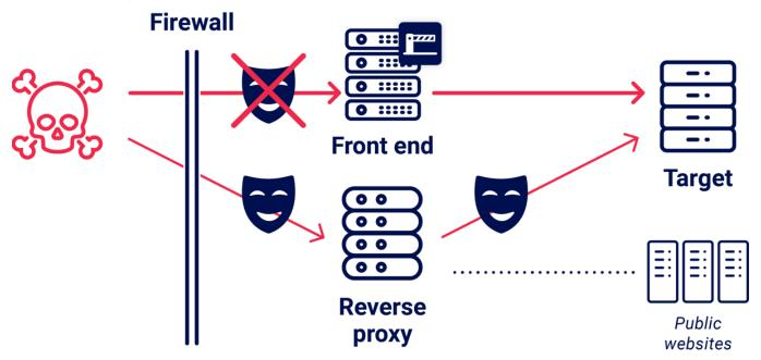
The easiest way to bypass this defense is to simply talk directly with the back-end, but this is usually impossible due to network firewalls. Another approach is <u>HTTP request tunneling</u>, which I used to <u>completely compromise New Relic's</u> <u>core internal API</u> using a header called "Service-Gateway-Is-Newrelic-Admin". You can also try <u>obfuscating headers</u> to smuggle them past the front-end.
