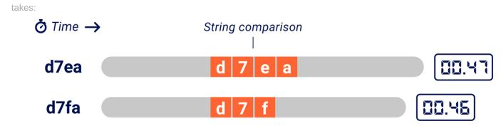
In this illustration, we're using two HTTP requests to ask the question 'Does the database contain a password reset token starting with d7e?' The server is taking one second to compare each character, so by comparing the response times an attacker can tell that the token starts with 'd7e' rather than 'd7f.
