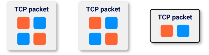
Unfortunately, this introduces a different catch - some servers start to process HTTP requests as soon as they've got the headers, without waiting for the body. To fix that, we need to persuade our OS network stack to coalesce the header frames into a single packet so that regardless of which stage the server starts processing at, both requests get processed at the same time:
