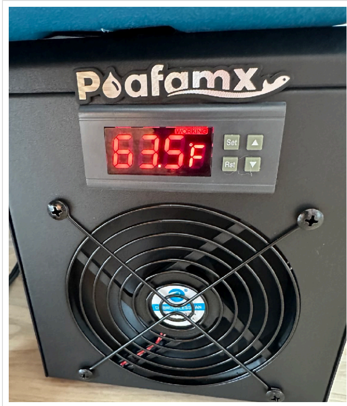
An image of the cooler used – I keep it set to as low as it will go which will usually be around 12°F lower than the air temperature.
