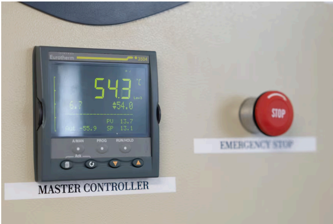
On this day, the climate chamber is set to an air temperature of 54C with 26 per cent humidity. (ABC News: Jack Fisher)
