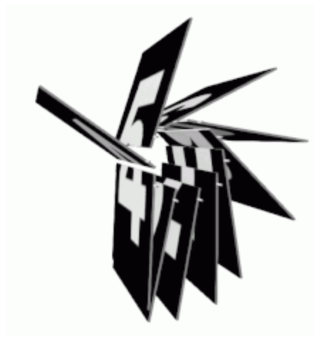
An animation of how a split-flap display works
