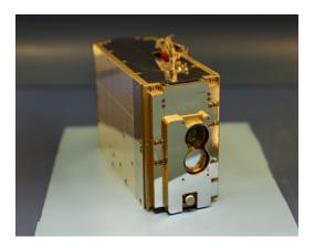
The TBIRD communications payload, pictured above, is showcasing unprecedented data rates for space-to-ground laser communications. Photo courtesy of Lincoln Laboratory.
