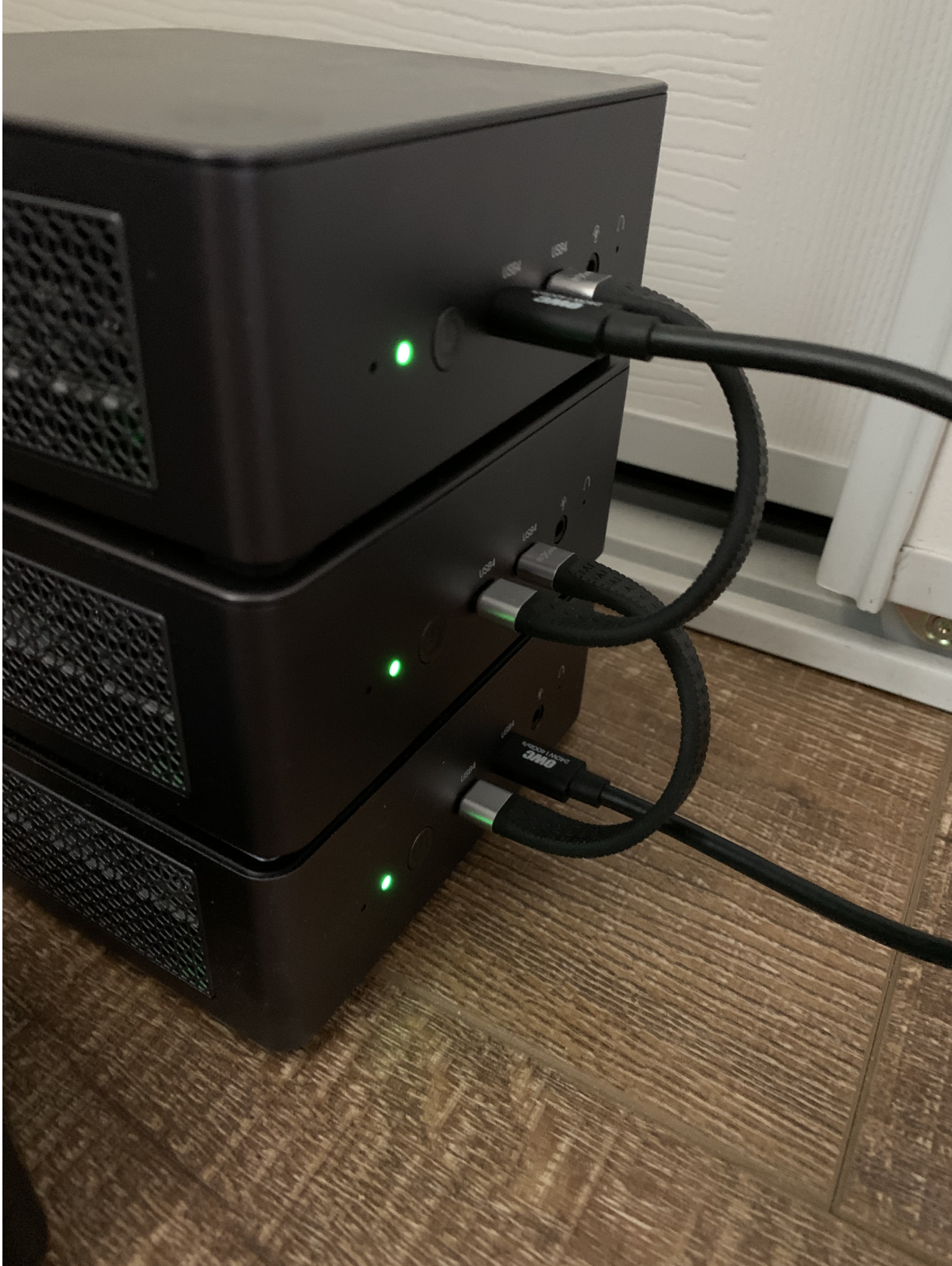
The UM790 Pro bare-metal cluster with full-mesh USB4 cables connections
