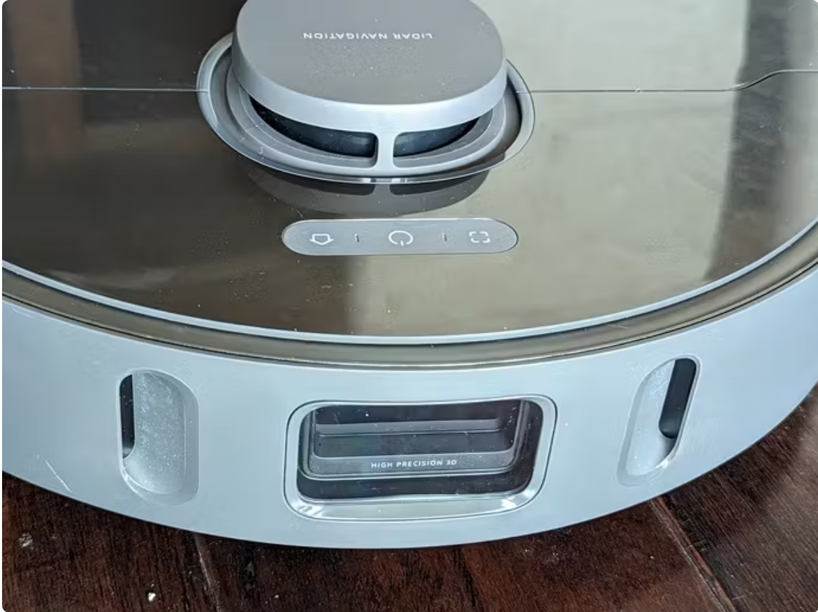
The lidar and front sensor cluster on the Z10 Pro. The robot shoots lasers out of the angled apertures, and an IR camera cluster in the center uses distortion in the beam to sense obstacles.
