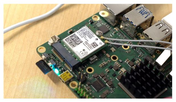
I also wanted to test the top A+E key M.2 slot. It's perfect for WiFi and I had an Intel AX210 I recently tested to 1.5 Gbps on the Raspberry Pi.
