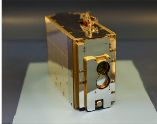
The TBIRD communications payload, pictured above, is showcasing unprecedented data rates for space-to-ground laser communications.
